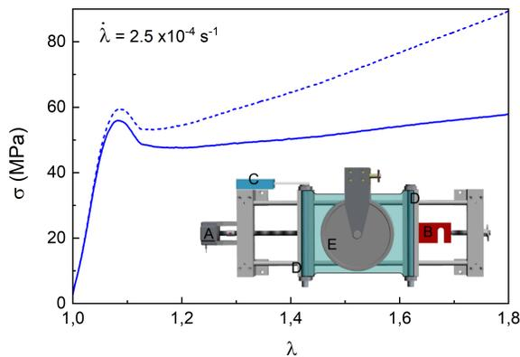
FIG. 1. Nominal stress (solid line) versus strain. Measured Young's modulus:  $G' = 817 \text{MPa}$ . An estimation of the true stress (dashed line) is also indicated, see discussion. Inset: Sketch of the experimental setup. (A) motor, (B) cell load, (C) linear actuator, (D) sample fastening cylinders, and (E) electrodes for the dielectric measurement. The whole setup is enclosed in a Faraday cage to minimize low frequency electromagnetic perturbations coming from the outside.
