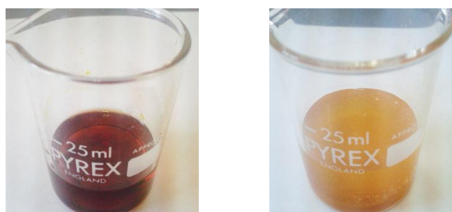
Figure S6. Mixture of both \text{FeCl}_3 and C solutions (left) and same mixture evolution after stirring (right).
