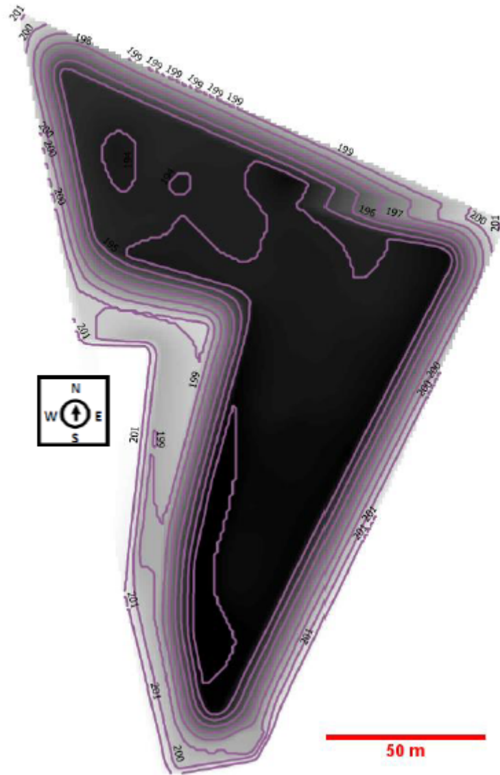
Fig.2. Topography of the Django Reinhardt infiltration basin: French projected coordinate system RGF93/Lambert 93 (in meter)
