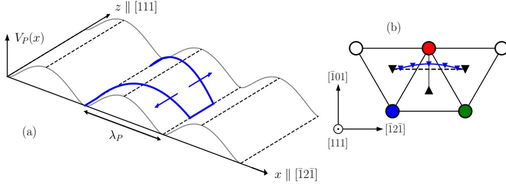
**Figure 16.** (a) Sketch of a dislocation line (blue) crossing a Peierls barrier through the nucleation and propagation of a kink pair. (b) Projection of the  $1/2 [111]$  screw dislocation trajectory gliding in the  $(\bar{1}01)$  plane with the three most displaced  $[111]$  atomic columns represented in blue, red and green.
