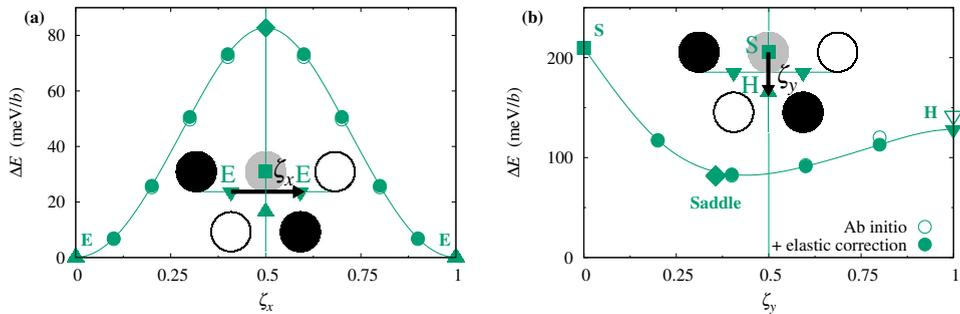
**Figure 3.** Energy variation of the dislocation along different paths in BCC tungsten [43]: (a) Peierls barrier, *i.e.* minimum energy path between easy cores; (b) Straight path between split and hard cores. The saddle configuration in (a) is also indicated by a diamond in (b). The insets show the path directions with the corresponding reaction coordinates,  $\zeta_x$  and  $\zeta_y$ .
