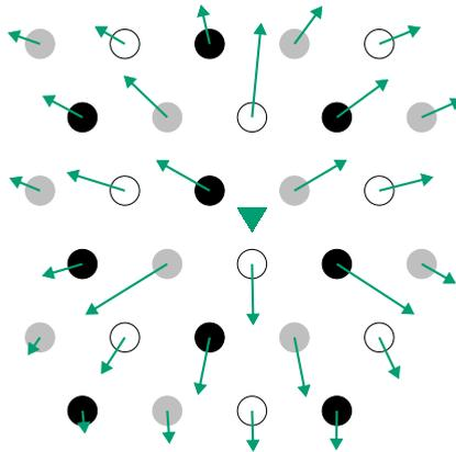
**Figure 8.** Atomic displacements in the (111) plane perpendicular to the dislocation line induced in BCC tungsten by the core dilatation of a screw dislocation in its easy core configuration. Displacement vectors have been magnified by a factor 50. The dislocation position is indicated by a downward triangle.
