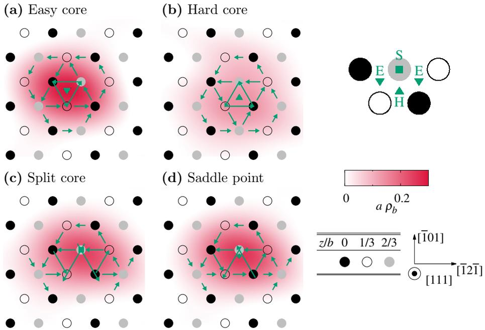
**Figure 2.** Core structures of a screw dislocation in BCC tungsten [21, 43]: (a) easy, (b) hard, (c) split cores, and (d) saddle configuration. The centers of the dislocation are indicated by colored symbols and are sketched in the right panel. Differential displacements and Nye tensors are shown as in Fig. 1.
