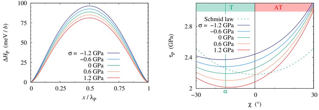
**Figure 10.** Dependence of the Peierls enthalpy barrier (left) and yield stress (right) on a non-glide stress  $\sigma$  perpendicular to the MRSSP (*cf* Eq. 16 for the stress tensor definition).  $\chi$  is the angle between the MRSSP and the  $\{110\}$  glide plane and is null in the left figure.
