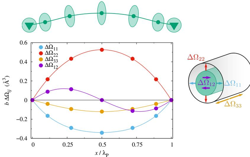
**Figure 9.** Variation of the relaxation volume tensor along the minimum energy path between easy core configurations. The different tensor components are shown as a function of the dislocation position  $x$  along the glide direction normalized by the distance  $\lambda_p$  between Peierls valleys. The corresponding shape of the 2D Eshelby inclusion along this path is sketched in the upper part.
