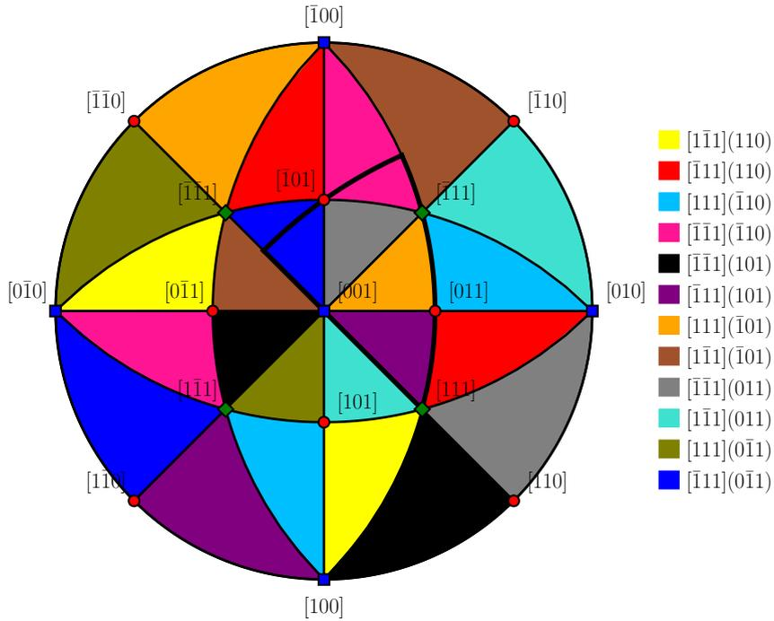
**Figure 12.** Stereographic projection of the BCC lattice showing in colors the regions where each individual  $\langle 111 \rangle\{110\}$  slip system has the highest Schmid factor. The thick black triangle is the minimum irreducible zone of the  $[111](\bar{1}01)$  slip system with  $\zeta \in [0, 90^\circ]$  and  $\chi \in [-30^\circ, 30^\circ]$ .
