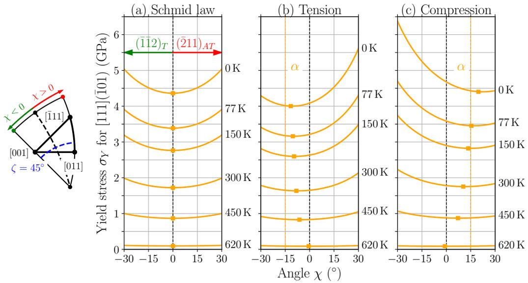
**Figure 19.** Yield stress of the  $[111]\bar{1}01$  slip system predicted from Eq. 28 at different temperatures as a function of the angle  $\chi$  for  $\zeta = 45^\circ$ : according to Schmid's law (a) and including non-Schmid effects in tension (b) and compression (c). The angle  $\chi$  leading to a minimum yield stress is indicated by a square symbol. Parameters as in Fig. 18
