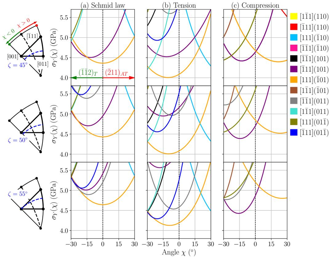
**Figure 14.** Yield stress of the different slip systems in tungsten under uniaxial loading at 0 K as a function of the angle  $\chi$  for  $\zeta = 45^\circ, 50^\circ, 55^\circ$ : (a) according to the Schmid law and including non-Schmid effects in (b) tension and (c) compression.
