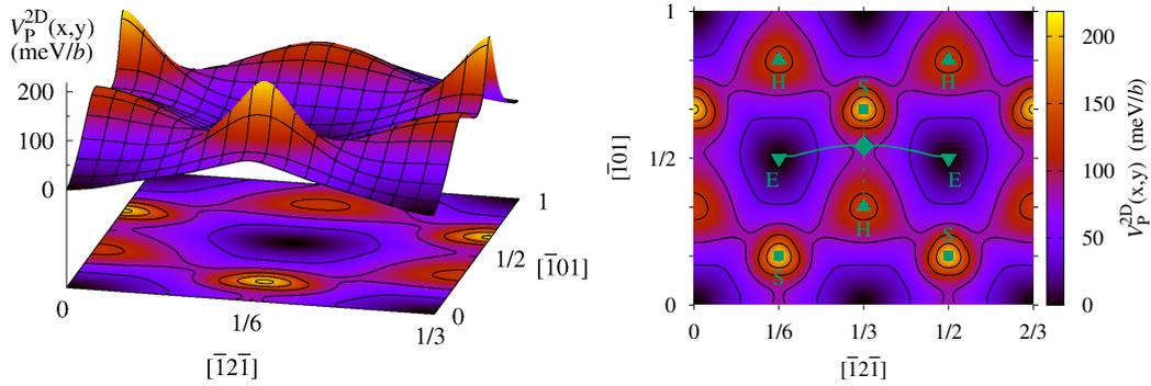
**Figure 4.** 2D Peierls potential of the  $1/2 \langle 111 \rangle$  screw dislocation in BCC tungsten [43]. In the projection on the right, the dislocation trajectory corresponding to the minimum energy path corresponding to the minimum energy path between two easy cores (Fig. 3a) is shown with a green solid line, while the dashed green line links the split and the hard cores (energy variation shown on Fig. 3b). The green diamond corresponds to the saddle configuration.
