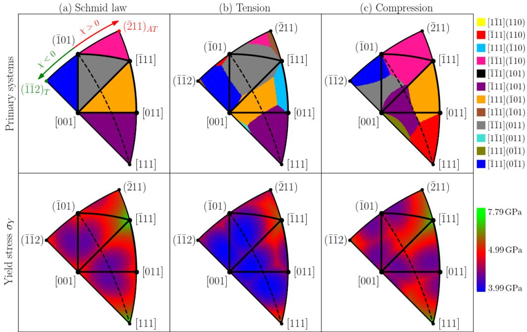
**Figure 13.** Primary  $\langle 111 \rangle \{110\}$  slip system (first row) and corresponding yield stress (second row) activated in tungsten single crystals under uniaxial loading at 0 K as a function of the orientation of the deformation axis and predicted using the Schmid law (a), and the yield criterion developed in this work in tension (b) and compression (c). The color coding of the different slip systems and the stress range are indicated in the legend on the left.
