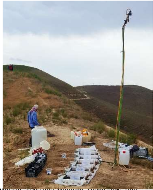
Fig. 2. Experimental setting for rainfall simulation in the Marzan-Abad and Miraven-Tapeh Sites, Iran
