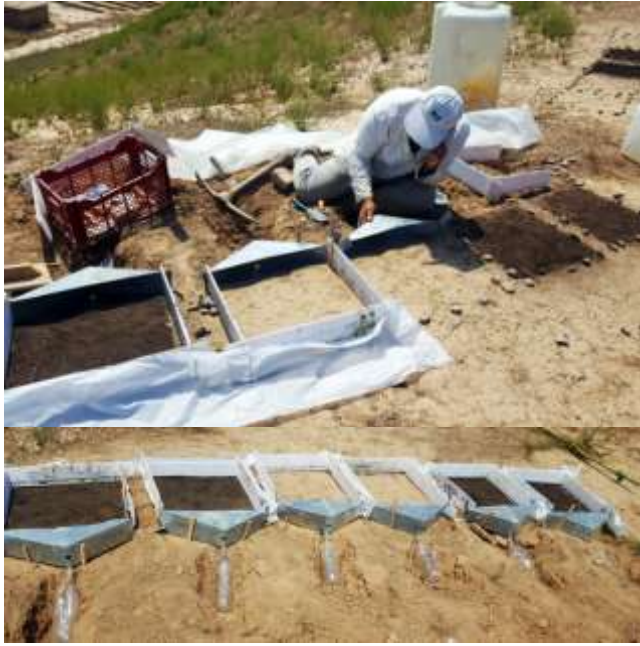
Fig. 2. Experimental setting for rainfall simulation in the Marzan-Abad and Miraven-Tapeh Sites, Iran
