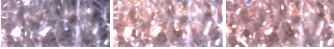
FIG. 6. Side view images (diffused reflected light) of the foam under 0 (left), 200 (middle) and 400 V (right) with a color camera ( L = 24 mm, R = 3 mm, image height is 20 mm.)
