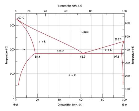
Figure 1. Pb-Sn phase diagram.
