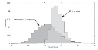
**Figure 14.** Comparison of model complexity of the trans-D model for the inversion with unknown STF (Section 4.2) and for the RF inversion (Section 4.3). Note that the uncertainty in the number of layers is much lower for the RF inversion. In addition, the RF inversion overestimates the number of layers which results in unreasonably complex shallow structure.
