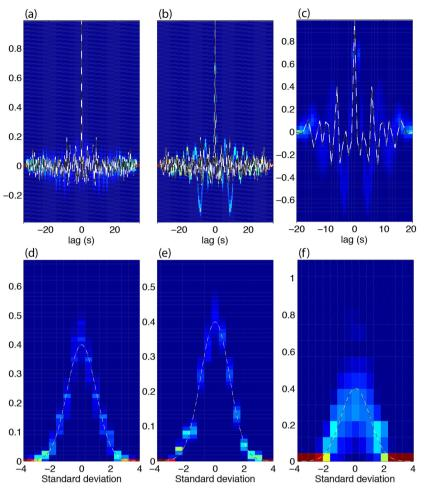
**Figure 10.** Residual analysis for HYB data in terms of autocovariance (a–c) and residual histogram (d–f) densities (colour) compared to simulated Gaussian (zero mean, unit standard deviation) densities (dashed). For (a, d) radial and (b, e) vertical components, and (c, f) SWD data.
