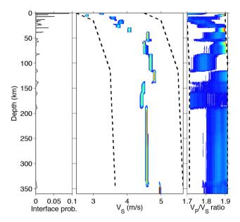
**Figure 12.** Receiver function inversion results (colour) in terms of profile marginal densities for station HYB and prior bounds (dashed). Note the much smaller (unrealistic) uncertainties than for the DSI result in Fig. 8.
