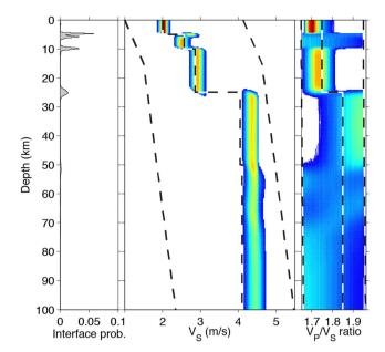
**Figure 4.** True earth model (dashed) and inversion results in terms of interface probability as a function of depth and profile marginal densities for  $V_s$  and  $V_p/V_s$  ratio. The extent of the uniform prior bounds are also shown (dashed).
