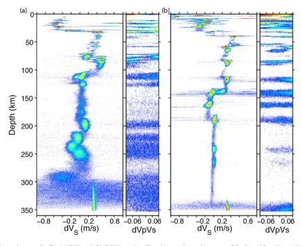
Figure 15. Comparison of inversion results for (a) DSI and (b) RF inversion. Results are shown in terms of the logarithm (base 10) of the perturbation position density. In (a), uncertainty increases with depth but the half-space is closely constrained due to the small errors on the long-period SWD data. In (b), uncertainty estimates are unrealistically small due to signal processing effects on data noise and since the RF inversion does not treat the STF as uncertain.
