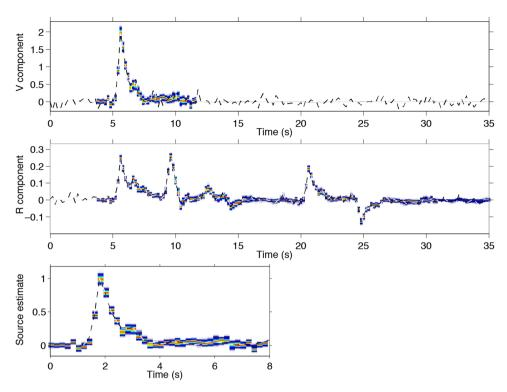
Figure 2. Noisy simulated waveforms (dashed) for (a) vertical and (b) radial components. The range of data predictions produced by the Bayesian sampling is shown as a density for each time sample (colour). Both waveforms are fit well in the inversion. (c) The true STF (dashed) and the probabilistic STF estimate (colour) closely agree.
