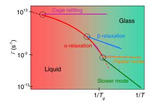
FIG. 4. Schematic Arrhenius diagram concerning dynamical behaviors of MG and its high temperature precursors. Data for  $\alpha$  and the  $\beta$  relaxations are from dynamical mechanical measurements on La<sub>55</sub>Ni<sub>20</sub>Al<sub>25</sub> MG (Fig. S3 [16]). The red line is the Vogel-Fulcher-Tammann (VFT) [3] fit to the  $\alpha$ -relaxation data and the blue line the Arrhenius fit to the  $\beta$ -relaxation data.
