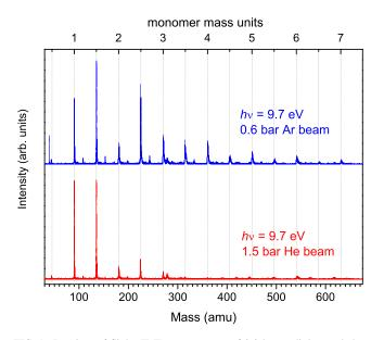
FIG. 1. Ion time-of-flight (ToF) mass spectra of 2,3 butanediol recorded at 9.7 eV photon energy in He and Ar molecular beam clustering expansions. An alternative mass scale calibrated in monomer mass units (1 monomer = 90.12 amu) is marked along the top axis.
