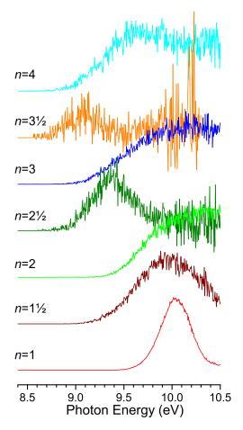
FIG. 3. Size-selected TPEPICO scans (size-selected TPES) taken in 0.6 bars Ar cluster beam conditions. The estimated threshold electron energy resolution was set as 50 meV to secure reasonable statistics. The individual traces have been normalized.
