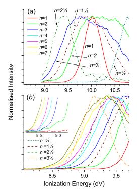
FIG. 4. VMI PES of individually normalised, size-selected 2,3-butanediol clusters recorded in (a) He clustering expansion (1.5 bars backing pressure) at hv = 11.0 eV; (b) Ar expansion (0.6 bars backing pressure) at hv = 10.0 eV. The inset here shows an expansion of the *n*-mer cluster threshold regions. The legends identifying cluster size apply in both panels.
