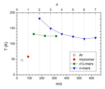
FIG. 5. Translational temperatures for ions produced in 0.6 bars Ar expansion and photon energy integrated from hv = 8.9-9.4 eV. The data were obtained by 3D ion momentum imaging using the DELICIOUS 3 spectrometer.<sup>9</sup>
