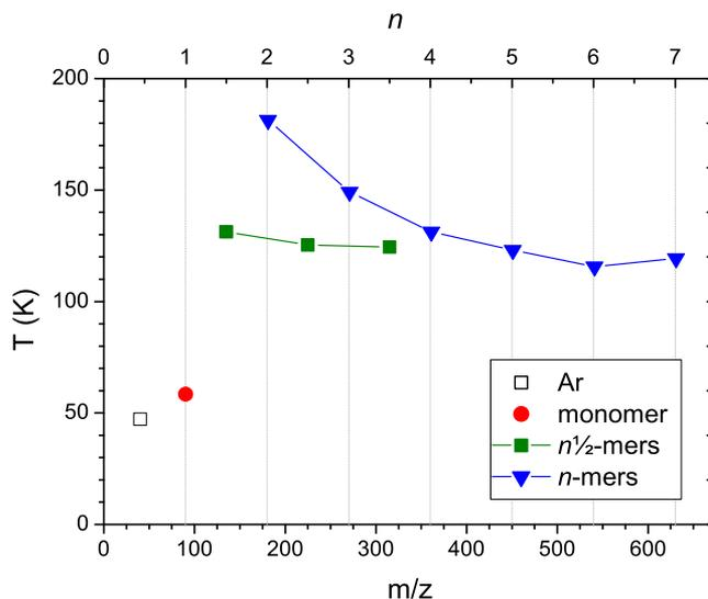
FIG. 5. Translational temperatures for ions produced in 0.6 bars Ar expansion and photon energy integrated from  $h\nu = 8.9-9.4$  eV. The data were obtained by 3D ion momentum imaging using the DELICIOUS 3 spectrometer.<sup>9</sup>
