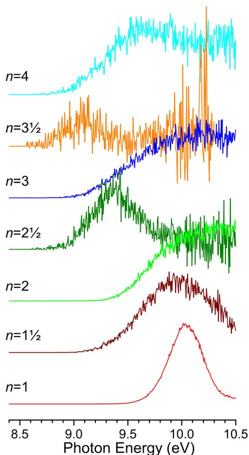
FIG. 3. Size-selected TPEPICO scans (size-selected TPES) taken in 0.6 bars Ar cluster beam conditions. The estimated threshold electron energy resolution was set as 50 meV to secure reasonable statistics. The individual traces have been normalized.
