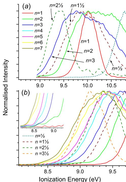
FIG. 4. VMI PES of individually normalised, size-selected 2,3-butanediol clusters recorded in (a) He clustering expansion (1.5 bars backing pressure) at  $h\nu = 11.0$  eV; (b) Ar expansion (0.6 bars backing pressure) at  $h\nu = 10.0$  eV. The inset here shows an expansion of the  $n$ -mer cluster threshold regions. The legends identifying cluster size apply in both panels.
