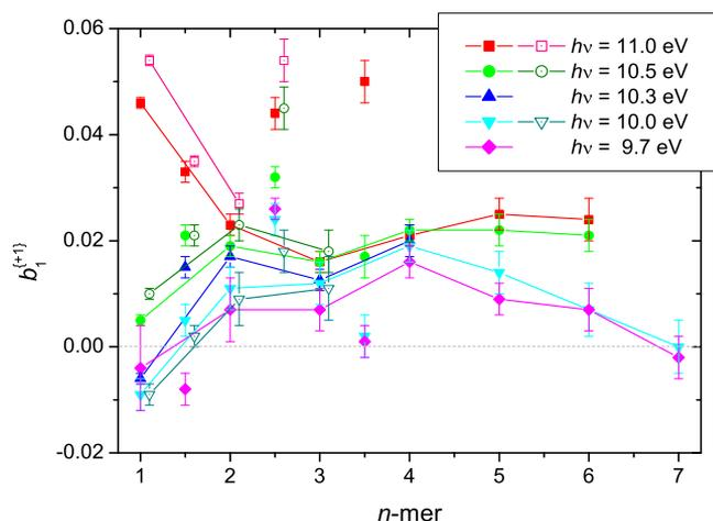
FIG. 6. Size-selected PECD  $b_1^{(+1)}$  parameters obtained as a weighted average over the associated VMI-PES band profiles. Straight lines joining the  $n$ -mer sequence values at a given photon energy are drawn to guide the eye, and exclude the  $(n + 1/2)$ -mer results. Measurements made in a 0.6 bars Ar expansion are plotted as solid symbols, those in 1.5 bars He with open symbols. The latter have been slightly displaced to the right for clarity.
