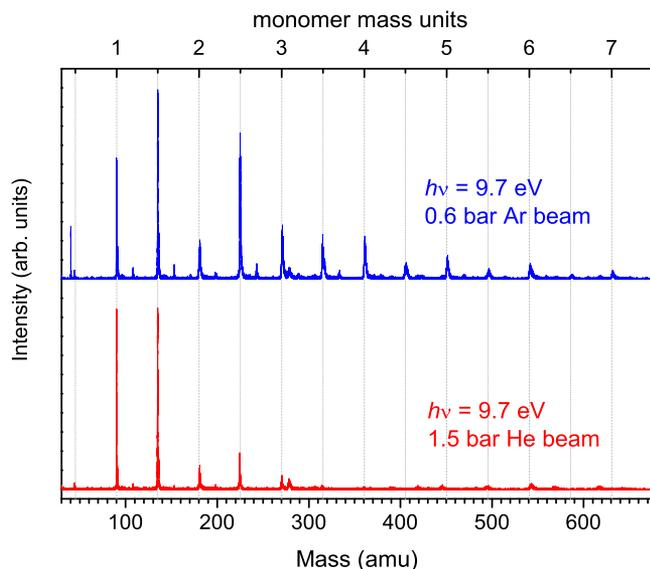
FIG. 1. Ion time-of-flight (ToF) mass spectra of 2,3 butanediol recorded at 9.7 eV photon energy in He and Ar molecular beam clustering expansions. An alternative mass scale calibrated in monomer mass units (1 monomer = 90.12 amu) is marked along the top axis.
