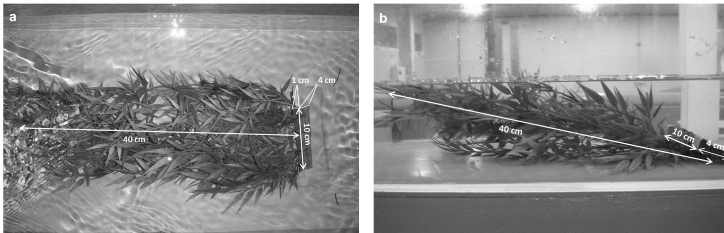
Figure 1. Pictures of the artificial macrophyte design in a hydraulic flume: (a) top view and (b) side view.
