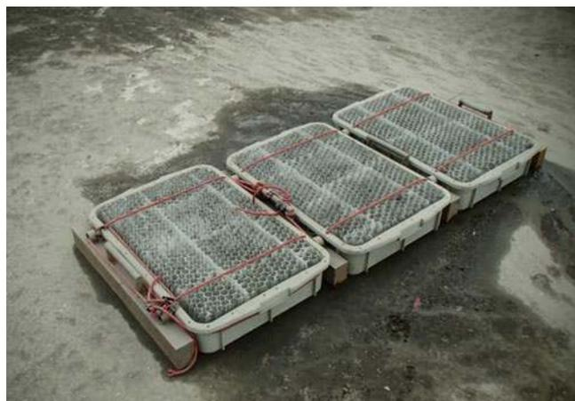
Figure 3. Photo of sediment traps.
