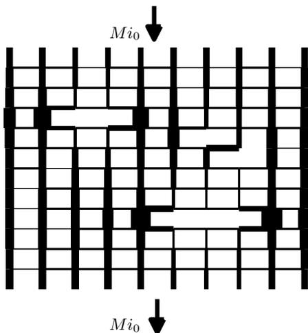
**Fig. 1.** Scheme of the 2D RFN on a square lattice. A total current  $Mi_0$  is applied at the top of the system in the vertical direction. The intact horizontal (vertical) fuses are represented by horizontal (vertical) lines whose thickness is proportional to the local current  $i_l$ . No line is drawn for the broken fuses. Notice that in the vicinity of broken fuses a higher local current flows on the intact vertical fuses.
