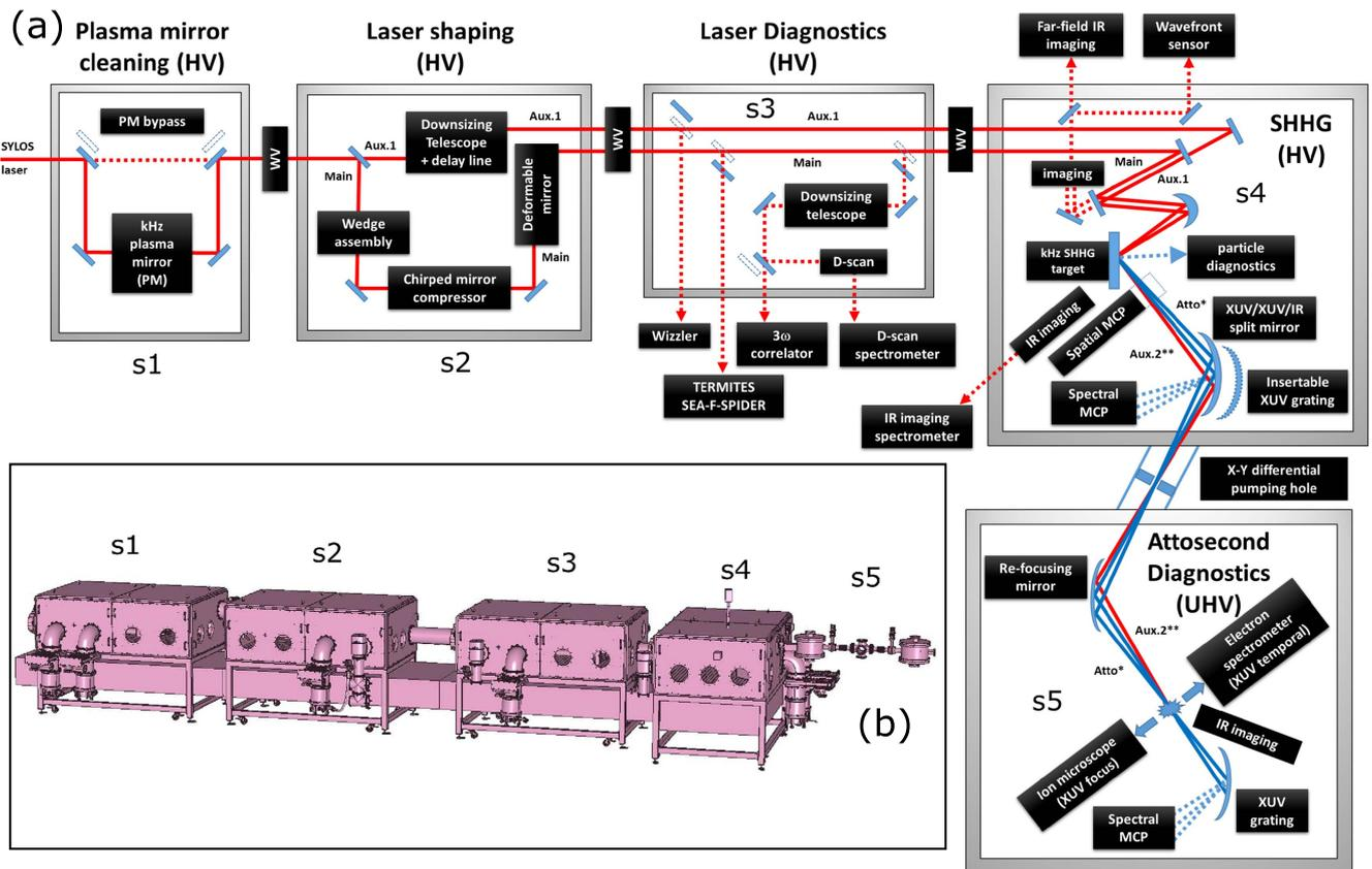
**Figure 30.** (a) Schematic optical layout of the beamline. (b) 3D view of the SHHG SYLOS beamline design showing the different sub systems s1-5. The SYLOS laser entry to the beam line is from the left of the figure.
