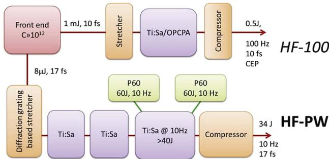
Figure 3. Block scheme of the HF laser system.
