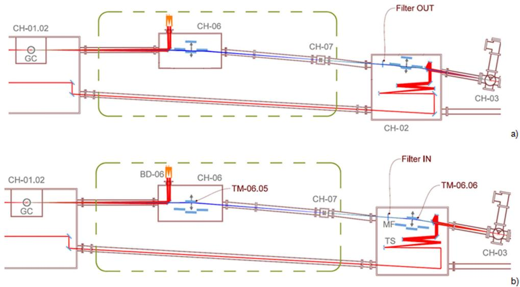
**Figure 11.** Geometry of the modified CONDENSED beamline to accommodate the double-stage grating monochromator: (a) monochromatic case; (b) broadband case. The section to be added (first stage of the monochromator and slit) is that within the dashed rectangle.
