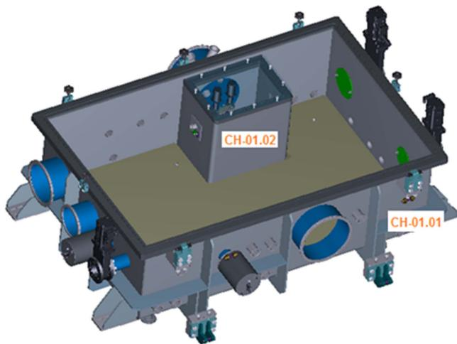
**Figure 10.** 3D layout of the main chamber of section 1. CH-01.01 hosts the optical elements and motorized movements to split and handle the two IR beams. The gas cell for the generation of attosecond pulses is hosted in CH-01.02, and is independently pumped to increase the differential pumping capabilities. The IR focusing mirror is mounted on an external chamber.
