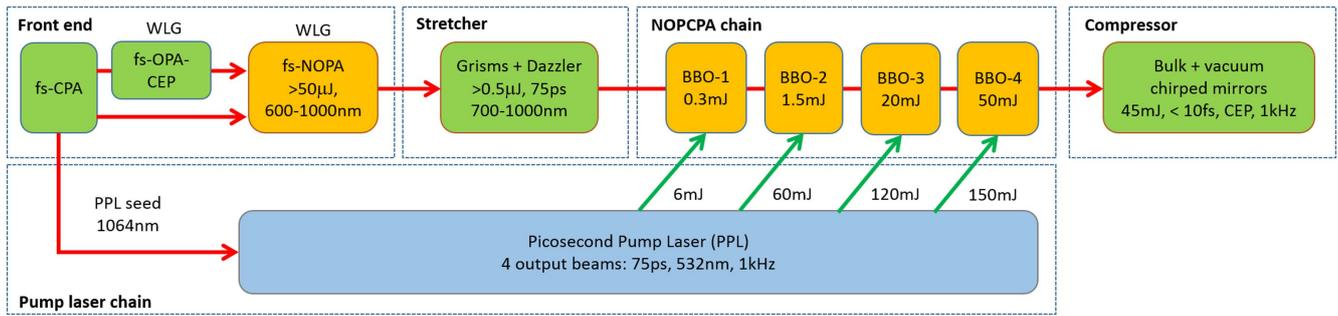
Figure 2. Block diagram for SYLOS 1 laser system.
