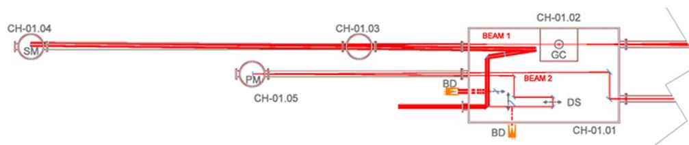
**Figure 9.** Optical layout of the section 1 of the two beamlines in phase 2. Two accessory chambers are added to the layout to host: respectively, a long-focal spherical mirror to generate XUV attosecond pulses, and a folding mirror to realize a longer path for beam 2. The subsequent sections of the beamlines are unchanged.
