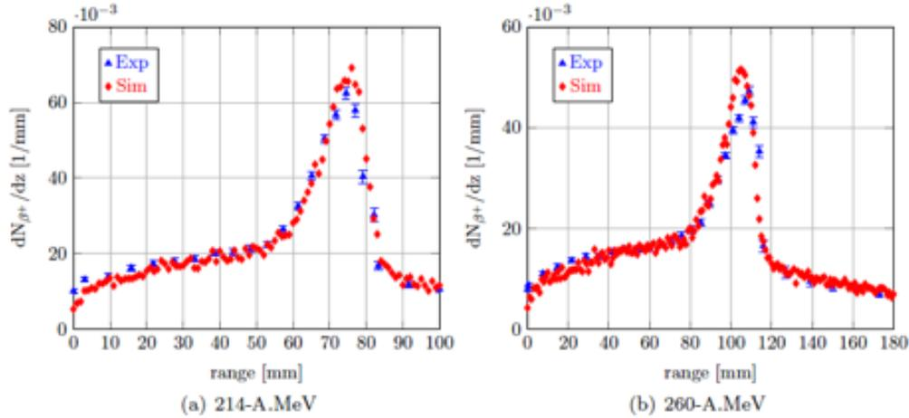
Figure 4.9: Experimental *versus* simulations: beta+-emitting isotopes depth profiles induced in a PMMA target by a 214 A.MeV carbon beam (a), 260 A.MeV carbon beam (b). Fiedler *et al* (2006), Priegnitz *et al* (2008, 2012)).
