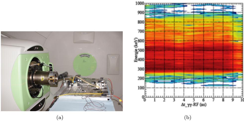
Figure 4.8: (a) Experimental setup at ICPO, with small acceptance LYSO detectors. (b) Energy *vs* Time distribution of coincidence events between the two detector heads. The beam pulse is 1 ns in length, with a period of 9.4 ns.
