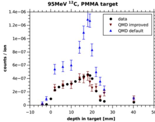
Figure 4.15: comparison between the prompt gamma profile measured at GANIL and simulations using various models in Geant 4 [DDDR<sup>+</sup>12].
