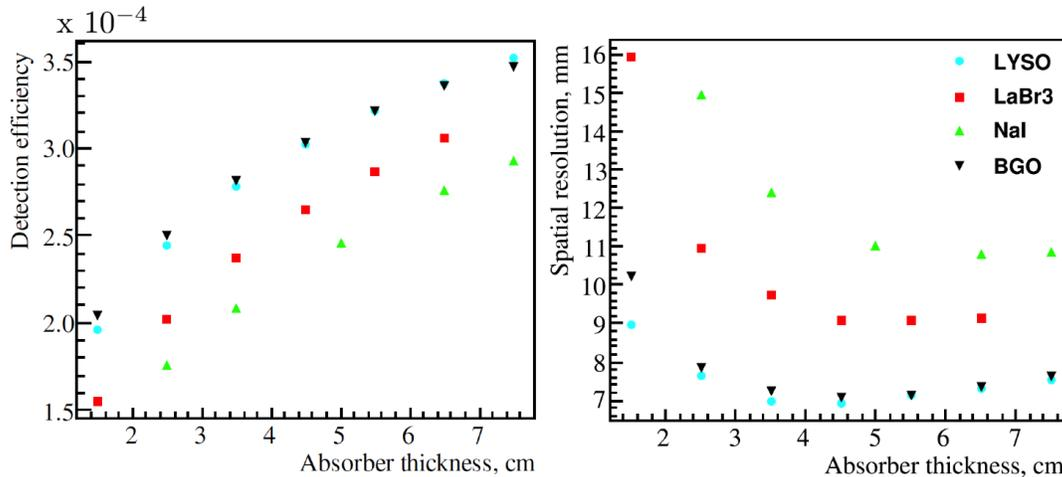
Figure 4.3: Simulation of a Compton camera performance according to the nature and thickness of the absorber scintillator [RDD<sup>+</sup>11].
