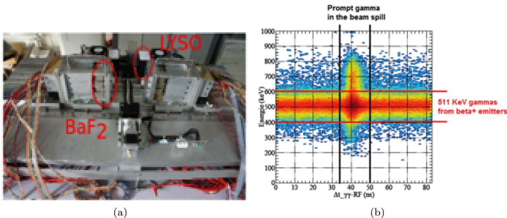
Figure 4.7: (a) Experimental setup at GANIL, with small acceptance LYSO and BaF<sub>2</sub> detectors. (b) Energy *vs* Time distribution of coincidence events between the two detector heads. The beam pulse is 1 ns in length, with a period of 80 ns.
