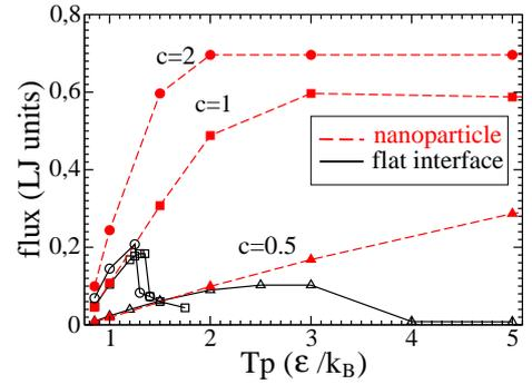
FIG. 4: Flux density as a function of the temperature of a nanoparticle (filled symbols) compared to the flux density flowing through a flat interface (open symbols). Lines are guides to the eye.
