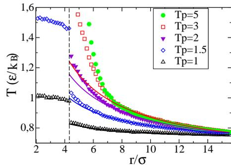
FIG. 2: Steady state temperature field across the liquid/nanoparticle interface, obtained with molecular dynamics. The nanoparticle/fluid interaction is hydrophilic ( $c = 1$ ). The position of the nanoparticle surface is indicated by dashed lines,  $r$  measuring the distance to the center of the nanoparticle. Solid curves correspond to fits by the continuum theory result  $T(r) = A/r + B$ . Note that for  $T_p = 1$ , the solid curve is indistinguishable from the simulation data.
